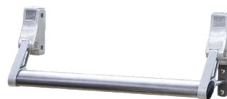
Anodized aluminum mounting plates and stainless steel latch cover, die-cast Zamak latch tongue, chrome plated zinc keypad housing, stainless steel inside push handle and strike
