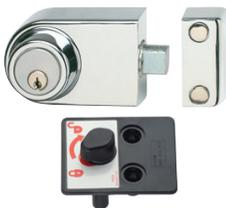
Die-cast Zamak exterior bolt housing and strike; 1" solid metal throw bolt; glass-filled, composite interior plate and thumb-turn; plastic thru-door shaft
