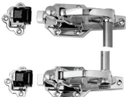
High pressure die-cast zinc body, forged brass handle and strike housing, forged steel tongue, malleable iron strike insert, stainless steel tube
