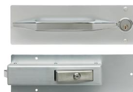
die-cast Zamak latch tongue, die-cast Zamak outside pull handle with polished chrome finish, stainless steel inside push handle and strike, nonconductive plastic couplings
