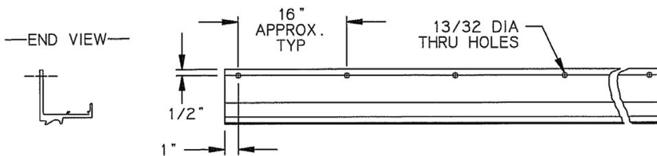
**Note:** Rail for 144" system is two piece rail. The track is used to align both sections.
