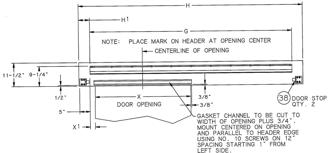
Fig. 9 shows a completed Header Assembly of a Manual Single Doorware System
