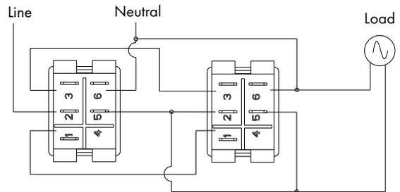
Three-way switch application indicator is "ON" when light is "ON"
