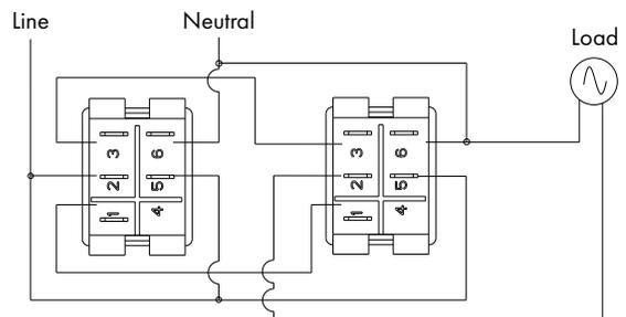
Three-way switch application "NIGHTLIGHT" or indicator always "ON"
