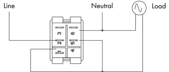
Single switch application indicator is "ON" when light is "ON"
