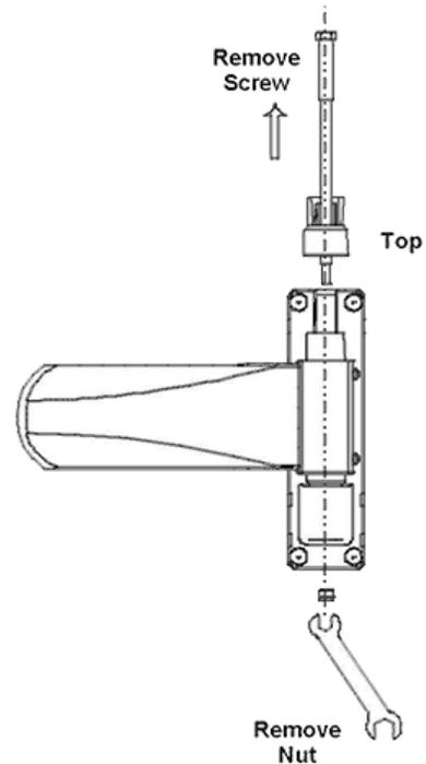
5. Open door and lift door clear of hinges as shown in Fig. 4 and Fig. 5.
