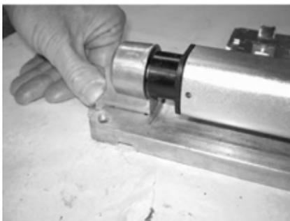
As nut is tightened top cap should move smoothly in slot
