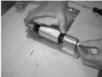
Put pressure on center screw to enable nut to start on threads
