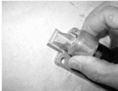
Slide top cap outward so that hex screw head seats fully within body
