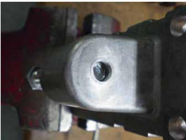
**Do not allow the bolt end to go past the cam material into the metal body of the hinge flange. Only a few turns into the cam material are required.**
