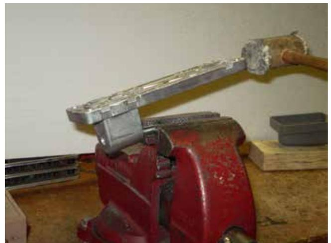
**Secure the bolt head in a vise, tap the flange body gently with a hammer.**
