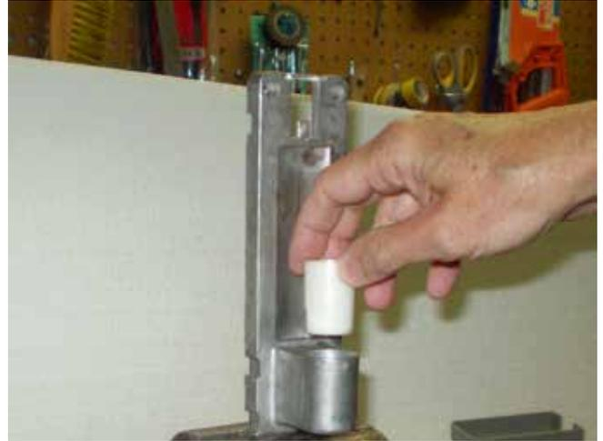
Place the new cam into the flange, indexing the flat side toward the back.
