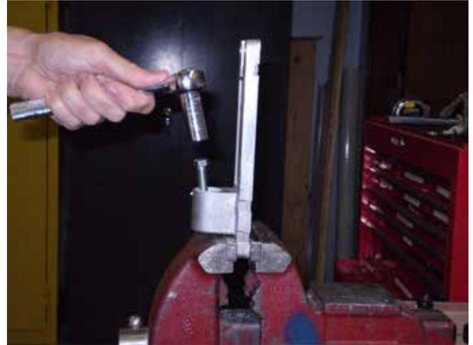
**Drive the bolt into the cam.**
