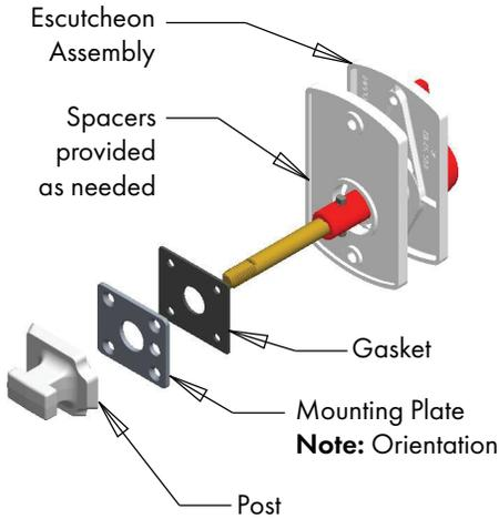
1. Mount handle on the door with the front mounting hole 2-7/32" from the edge as shown in the figure below.
