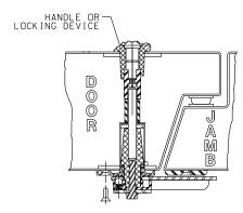
INSERT ENTIRE ASSEMBLY INTO RELIEF HOLE ON INTERIOR SIDE OF DOOR, ALIGN SQUARE ROD WITH SQUARE IN HOLDER PUSH TO FULLY SEATED POSITION
