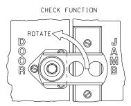
KEY SHOULD ROTATE LOCKING MECHANISM FREELY TO LOCK AND TO UNLOCK POSITION.
