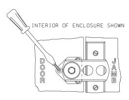
ORIENT INSIDE RELEASE MECHANISM AS SHOWN AND FASTEN IN 3 PLACES
