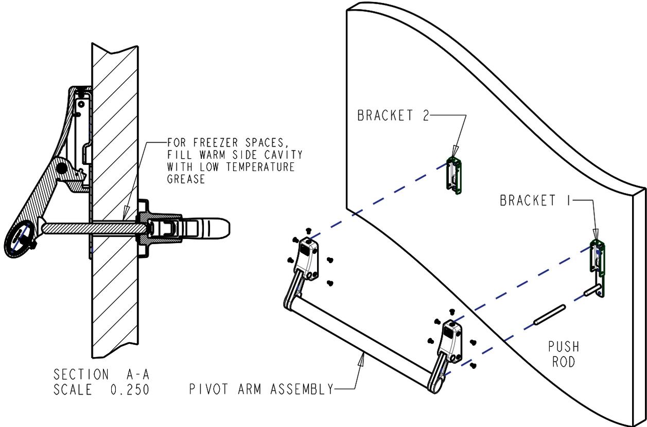
7. Secure pivot arm assembly with hardware provided, test function, use instruction sheet [IS-0778](#) to complete installation.
