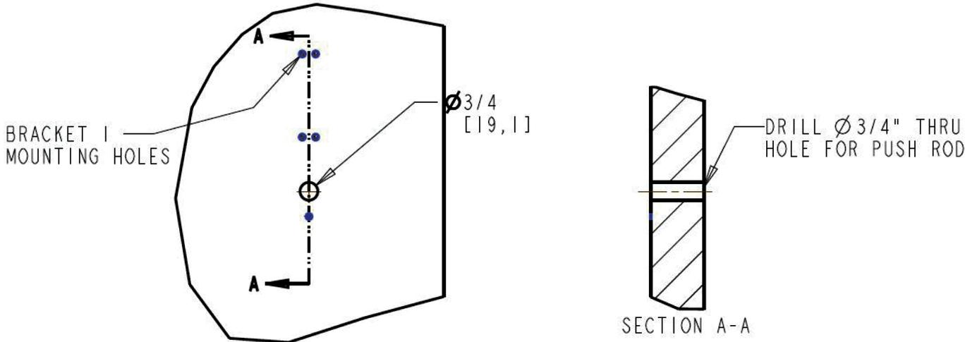
5. Install Bracket 1 and 2 with 1/4-20 structural hardware (not included).
